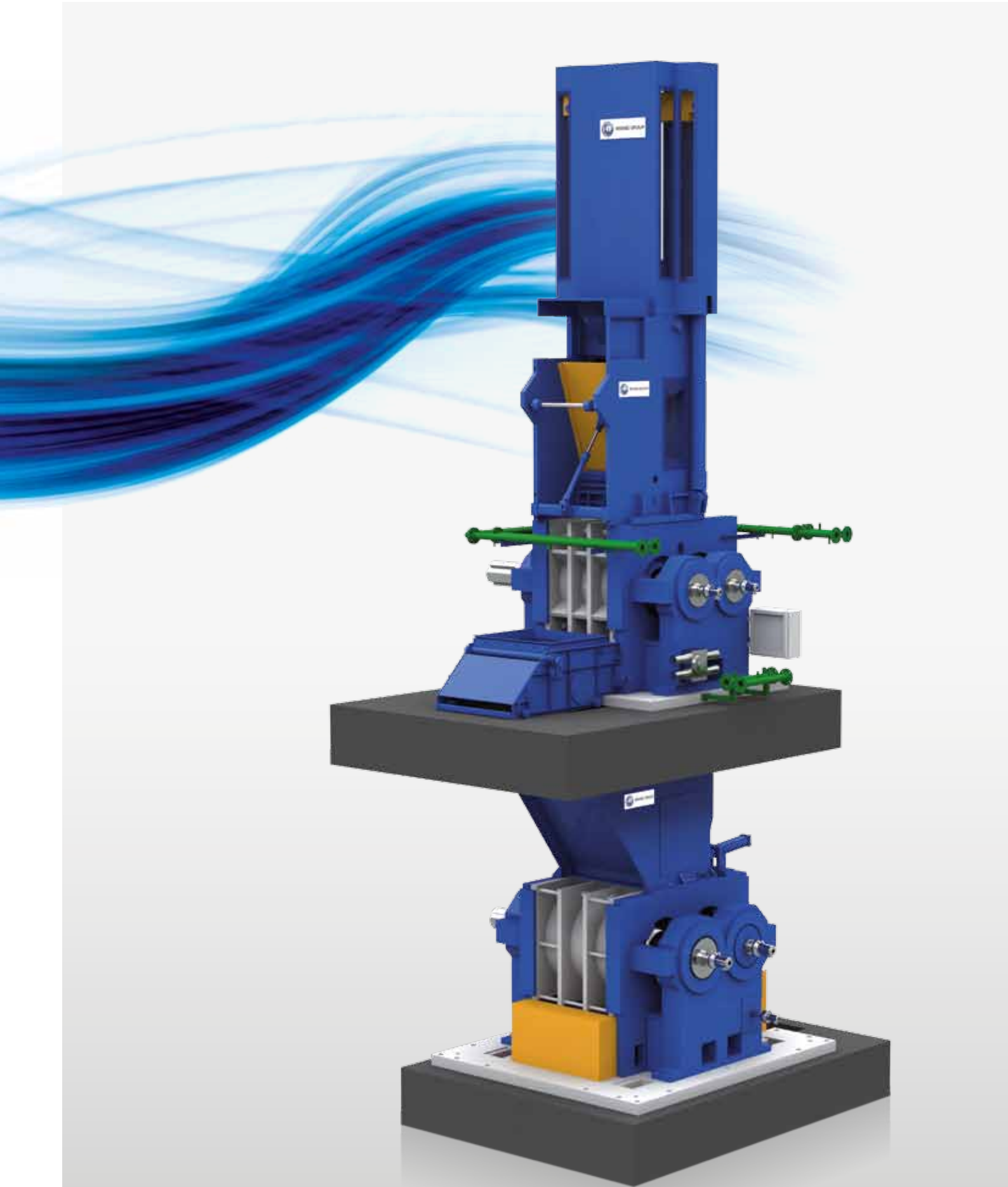
The basic principle behind the TANDEM mixer: the mixing stage (upper area) and kneading stage (lower area) work as an effective unit together.
